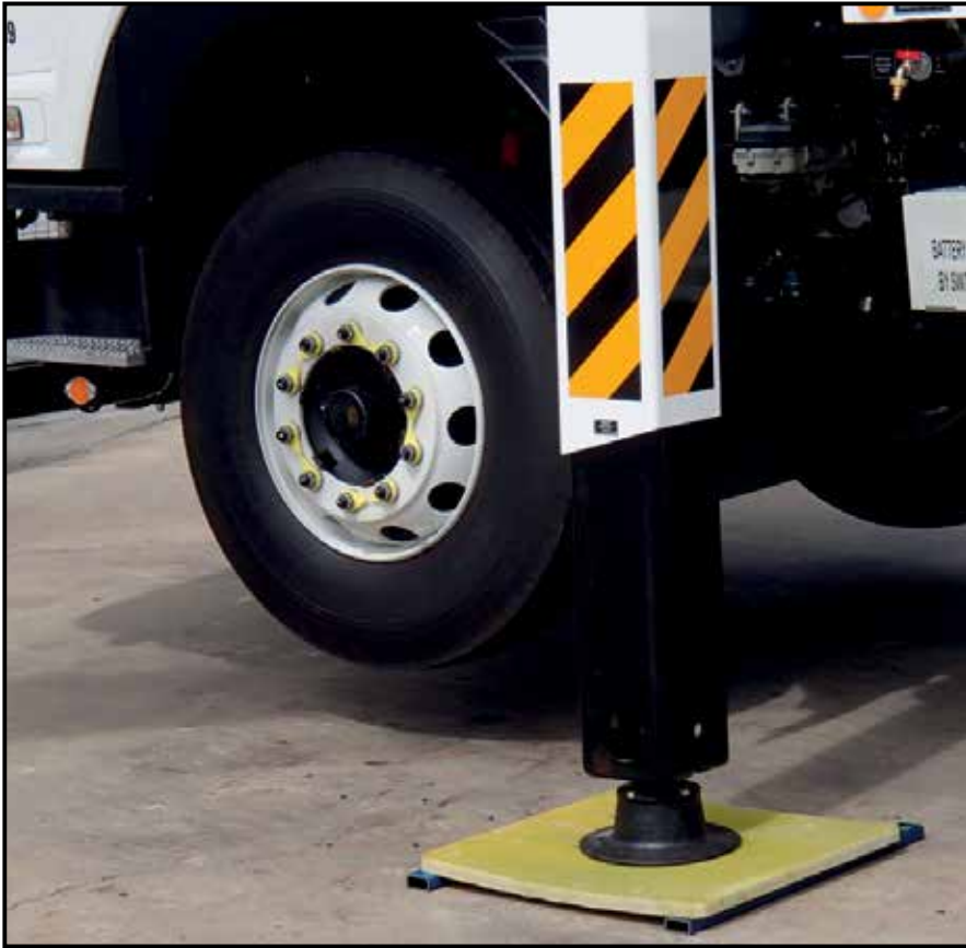
Dunnage supporting full test load of the truck over free span
