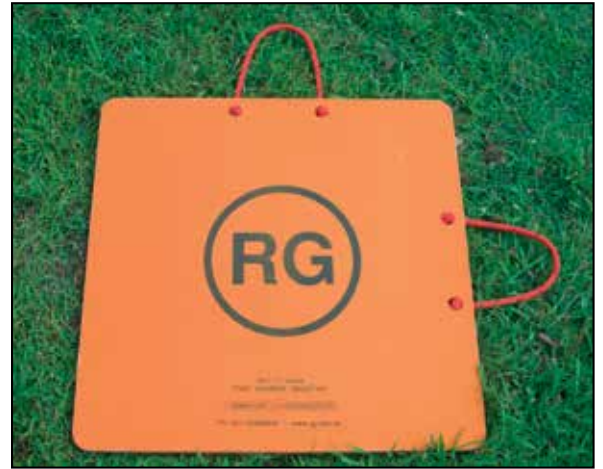
Recommended for MEWP or other mobile plant up to 14.5 tonne jackleg loads. 550 x 550 x 16mm
