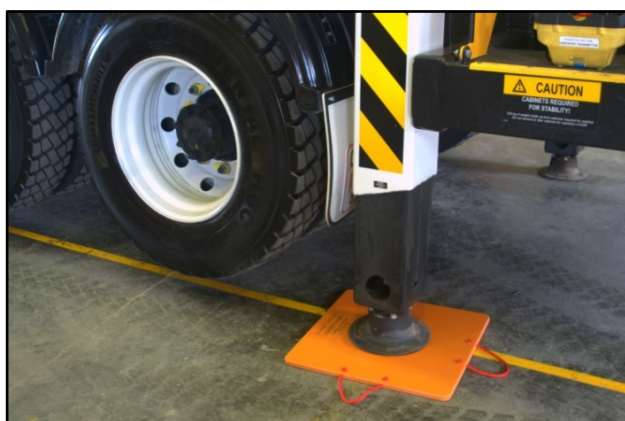
Figure 2 – Single Area with 1 RGA FRP Pads
