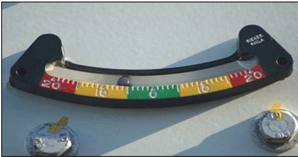
Figure 1 - Inclinometer depicting an out of operating range slope
