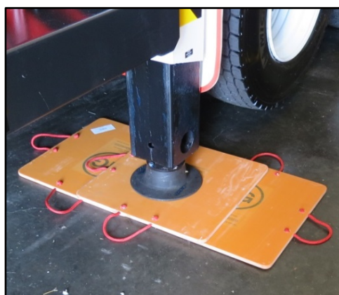
Figure 3 – Double Area, 3 RGA FRP Pads
