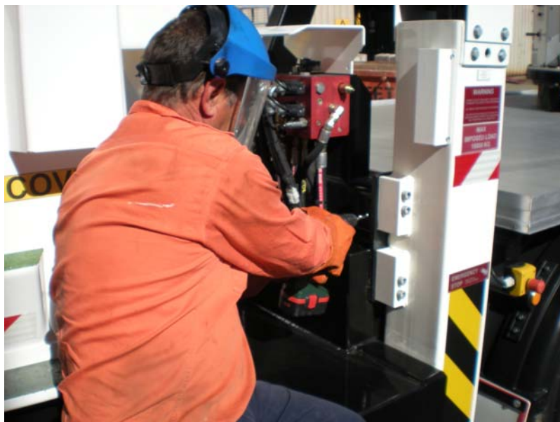
Hole being drilled in rear cross member
